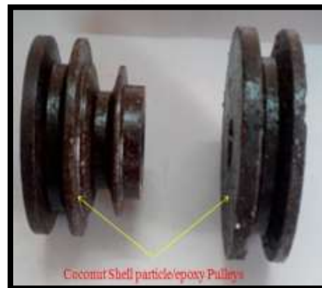
Figure 8(a). Geometry of Pulleys Figure 8(b). CSPE composite Pulleys Cylindrical composite pulley blanks for generation of pulleys were fabricated using cylindrical molds
