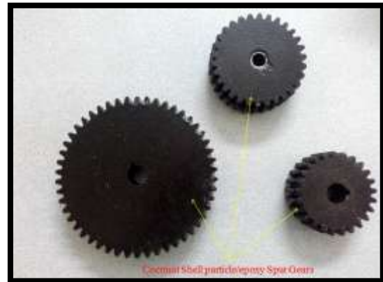
Figure 6. Generation of Gears using gear hob Figure 7. Generated CSPE composite Gears
