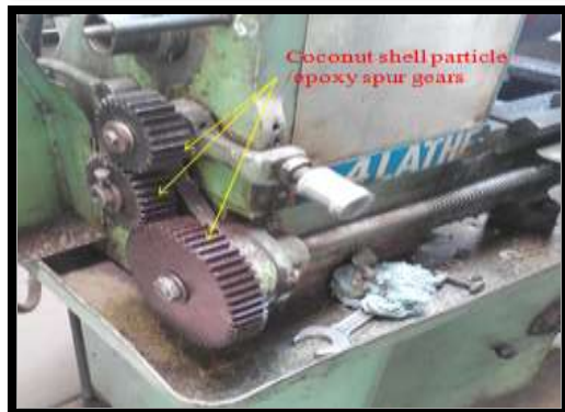
(a) Existing steel gears (b) Replaced composite gears
